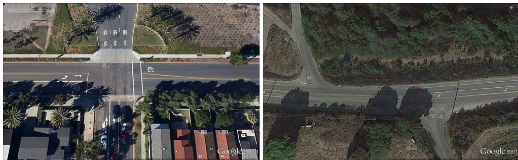
Fig. 3. Safer (left) and less safe (right) unsignalized intersections.
